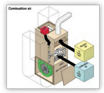
HIGH EFFICIENCY Some high efficiency furnaces **FURNACES** bring outside air for combustion directly into the burner through
