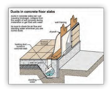
OTHER DUCT Common problems with supply ducts and registers are disconnected or obstructed ducts, PROBLEMS dirty ducts, ducts sized adequately for heating but inadequate for air conditioning, ducts sized for conventional furnaces, but inadequately sized for high efficiency systems, and unbalanced ductwork (too much air coming through one register and not enough air coming through another).
