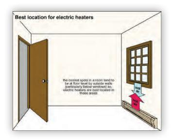
the baseboard heater. Heaters with fans can also be installed in the floors, walls and ceilings, for example. The best place for a heater is in the coolest part of the room.
