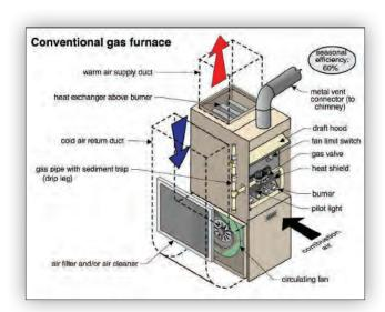
normal operation, the average seasonal efficiency of a conventional boiler or furnace is about 55% to 65%. That means 35% to 45% of the heat from the fuel is lost. With the advent of more efficient furnaces and boilers, this system became known as a conventional system. Conventional systems were phased out in the early 1990s.
