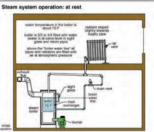
**ONE-PIPE** A one-pipe steam system has a **SYSTEMS** single pipe attached to each radiator. Steam moves through this pipe to the radiator, and the condensate flows back to the boiler through the same pipe. One-pipe systems cannot be converted to a hot water system without the addition of a second pipe.
