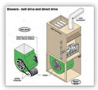
motors (ECM or Electronically Commutated Motors) are more efficient (use less electricity), but are more expensive than traditional (PSC or Permanent Split Capacitor) motors. ECM motors have the additional advantage of a larger range of operating speeds than conventional motors.
