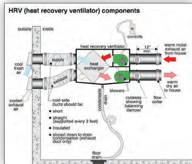
**FRESH AIR DISTRIBUTION** The fresh air coming into the home is filtered and then usually dumped into the return air ductwork for the furnace and mixed with the rest of the air. This distributes fresh air to all parts of the house.
