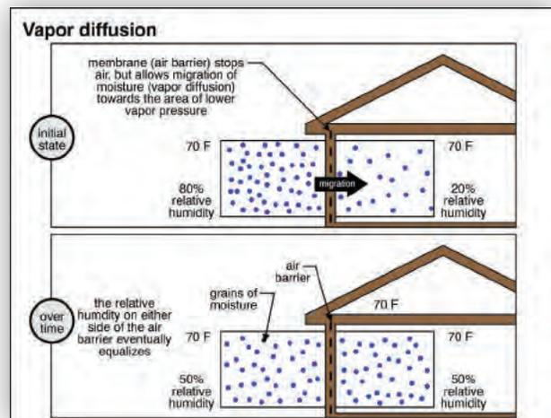
In warmer climates, where air conditioning is more dominant than heating, vapor barriers are not used, because a vapor barrier in the inside of the insulation can cause problems during the cooling season. Even in cold climates, vapor barriers are not as important as air barriers.
