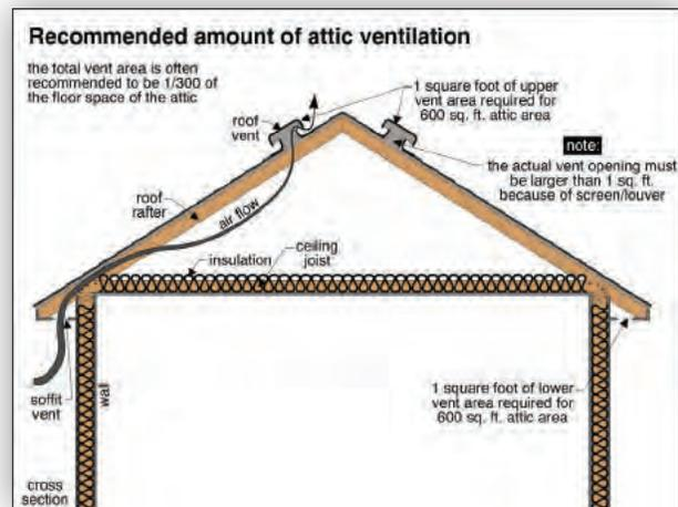
**VENT LOCATION** Roof vents (the common round or square metal vents) and/or gable vents should account for 50 to 80% of the total venting. They should have screens to keep insects and birds out of the attic. They are often located high on the downwind side of the house to help create a draft up through the eaves. The remaining ventilation is provided at the eaves. Baffles are used to keep soffit vents clear of insulation. On some houses, soffit venting is not practical.
