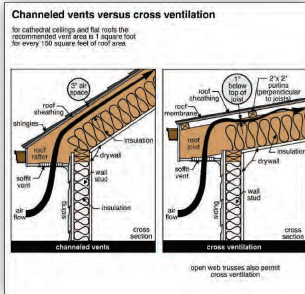
**ALTERNATIVE TO VENTILATION** Filling the cavity with an insulation that acts as an air and vapor barrier may be practical. The thought here is that if the roof space is sealed, warm moist air from the house can't get into the roof space and condense.
