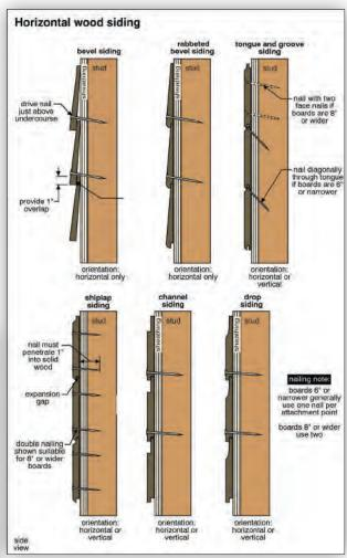
Water penetration and rot problems are most common at joints, penetrations and changes in direction or material. Joints should prevent water penetration. The horizontal joints on clap-board siding, for example, overlap one another; however, most vertical joints do not. Therefore, vertical joints should be protected with flashings or caulking. Caulking is a maintenance issue.
