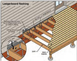
ROT Trapped moisture in a porch or deck structure rots wood beams or joists, weakening the structure and providing an ideal environment for insects. Many porch beams are concealed in a roof structure and are not visible, but years of roof leaks cause beams and joists to rot and the roof system to sag.
