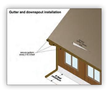
MATERIALS Gutters can be made of several materials; however, the most common are aluminum, galvanized steel, plastic and copper. Integral gutters are usually framed in wood, and lined with metals such as lead or copper. There are advantages and disadvantages to the various materials used.
