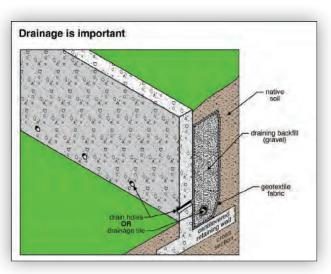
Minor repairs to retaining walls can be done by the homeowner. Patching cracked concrete retaining walls allows for monitoring of future movement. Major retaining wall repairs or modifications should be left to an expert. Retaining walls are often poorly built and can be very expensive to repair or replace.
