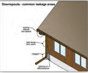
LOOSE Gutters and downspouts may become loose and require re-securing. This is normally due to improper fastening during original installation or damage caused by snow and ice during winter months. Downspouts can become disconnected from gutters.
