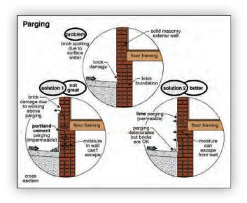
based parging prevents this phenomenon from happening as moisture can pass through it. The parging itself is subject to efflorescence and spalling, but this is treated as sacrificial material.
