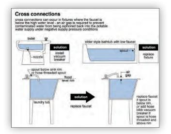
BIDET IS Some plumbing fixtures neces-ACCEPTABLE sarily create a situation which could lead to a cross connection. A bidet is a good example of this. A bidet has a water supply at the bottom of the bowl. This allows water to be directed up in a spray from the bottom center of the bowl. There is, of course, the potential for waste water in the bowl to get into this supply water. A special device (vacuum breaker) prevents water from flowing back into the supply plumbing.
