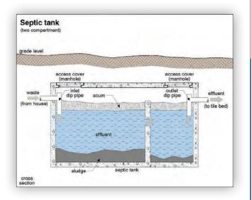
Most of the material entering the tank is in a liquid state. Within the tank, the majority of the solids are broken down to gases and/or liquids. The breakdown takes place as a result of bacterial action, both aerobic and anaerobic. The liquids are discharged from the tank into the tile bed. The gases escape through the plumbing vents in the home.
