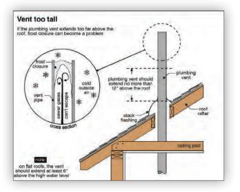
**CONNECTION/** Since the venting system only carries air, leakage is usually not a big problem. Deterioration of **PIPE SUPPORT** the piping is also very unusual, although poor connection or poor pipe support is a possibility.
