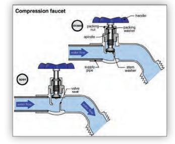
leaking washer will only allow water to drip into the fixture, while leaking packing will allow water to run onto a counter top, where it may cause damage.
