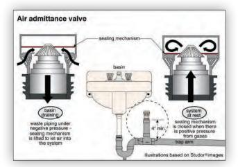
**AUTOMATIC AIR** While air admittance valves are **VENTS** approved in some areas, older style automatic air vents (see illustration), which rely on metal or rubber components, are not approved and should be replaced.
