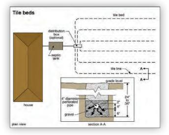
that are pumped out on a regular basis. There are also sophisticated systems with agitators and aerators that accelerate the chemical decomposition of the solids in the tank. These systems allow for smaller tile beds and are useful on smaller properties. While there is an advantage to this, the complexity of electrical and mechanical parts creates the potential for higher maintenance.
