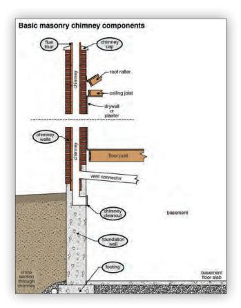
FLUE LINERS Some flues have masonry exposed on the inside. Unlined chimney flues are common in houses built before 1940. These unlined masonry flues often work well for fireplaces and oil-
