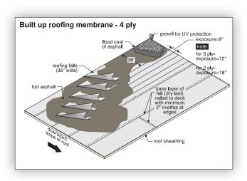
mechanical damage. These roofs are still common commercially, but are being replaced residentially with newer systems that are faster and easier to install.
