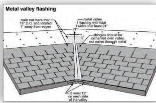
Sometimes a valley flashing is installed and then covered with shingles. This is called a closed valley. These may be closed cut or fully woven.
