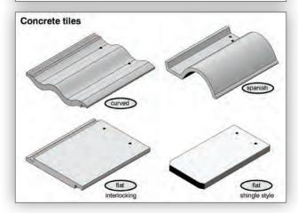
FASTENING Some systems are nailed in place while others use special clips or wire ties. In some regions, the tiles are mortared into place. In areas prone to high winds and hurricanes, these heavy tiles can be torn off roofs, becoming dangerous projectiles.
