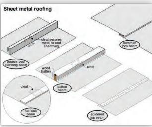
WEAR FACTORS Like any roofing system there are disadvantages; seams may split or be damaged. All metal roofs except copper and pre-painted or pre-coated roofs should be painted on a regular basis. Metal roofs should never be covered with tar because moisture trapped below the tar causes rusting. Tar covered metal roofs are usually near the end of their life. Metal roofs are difficult to repair and replacement is often the most practical alternative.
