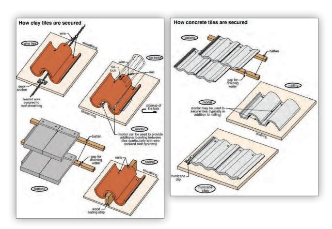
WEAR FACTORS Like any brittle roofing system, concrete and clay tiles are subject to mechanical damage, and like any long-lasting roof system, the fasteners may wear out before the tiles. Depending upon the design of the roof system, they can be very difficult to repair.
