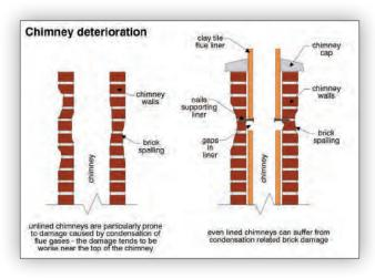
GAP IN LINER Some masonry chimneys lined with clay tile have a gap in the liner. The top flue tile should protrude two to four inches beyond the top of the chimney. If the top section of clay tile was
