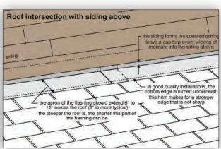
When the side of a roof ends at a wall, two sets of flashings are used. L-shaped step flashings are installed between each layer of shingles. The vertical part extends up the wall and is covered by siding or a metal counter flashing. Counter flashings are used on masonry walls, and the top may be let into mortar joints or sealed to the face of the masonry with caulking (a less permanent approach).
