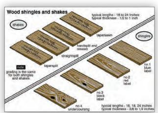
Wood shingles can be used on roofs with a slope as low as 3-in-12; however, 6-in-12 or more is recommended. Wood shingles vary in length between 16 inches and 24 inches. On a good quality installation, no more than one-third of each shingle is exposed to the weather.
